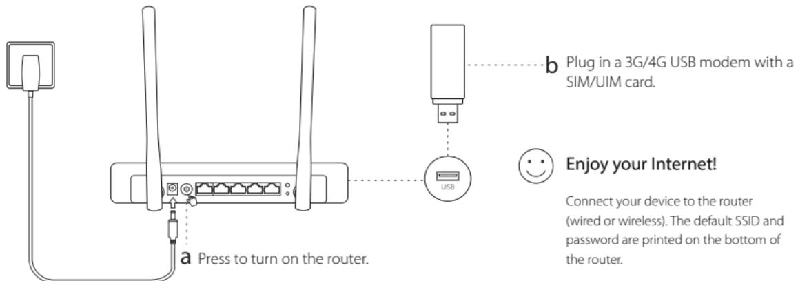
Connect your device to the router (wired or wireless). The default SSID and password are printed on the bottom of the router.
