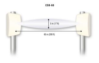
The microwave barriers consist of an invisible cigar shaped protection beam generated between the transmitter and the receiver installed in the protected area. The microwave barriers are suited to protect high risk installations such as airports, factories, military sites, etc.
