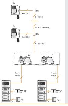
A KM8100W WB8600 B 1281E C 1473 D Mody The Video Intercom system of the Compact line, composed by the b/w flat or CRT monitors flush or surface mounted exploits the coaxial cable as transmission mean for the video signal. The electronic chime technology guarantees extra quality to the audio reducing any interference potentially on the line. It can be perfectly used with any FAR-FISA door stations and it is also available in video kit versions for one way systems.
