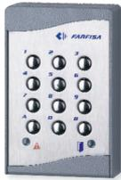
Access Control keypad IP45 surface mounted with stainless steel front plate and buttons. Two relays for lock opening, access control, etc. Keypad for programming and setting relay enable codes. Keypad deactivation with increasing time intervals (max 25 sec.) in case of wrong combination. Programmable codes up to 8 digits for each
