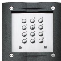
Anti-vandal stand alone keypad (IP45, with stainless steel front plate and buttons) that can be installed singularly or combining it with conventional or digital audio or video Matrix composition. It works with 2 relays for lock opening, access control etc. with 12 programmable codes from 1 to 8 digits for each relay.
