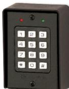
Access control keypad with front plate, buttons and box in plastic. One lock-opening relay, access control, etc. Keypad for programming and setting relay enabling codes. Keypad deactivation with increasing time intervals (max 25 sec.) in case of wrong combination. 8 programmable codes from 2 to 6 digits. Programmable timer from 1 to 99
