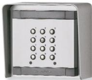
Access Control keypad with aluminium front plate and buttons in stainless steel. Two relays for lock opening, access control, etc. Keypad for programming and setting relay enable codes. Keypad deactivation with increasing time intervals (max 25 sec.) in case of wrong combination. 4 programmable codes from 2 to 6 digits for each relay.
