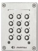
Access Control keypad with aluminium front plate and buttons in stainless steel. Two relays for lock opening, access control, etc. Keypad for programming and setting relay enable codes. Keypad deactivation with increasing time intervals (max 25 sec.) in case of wrong combination. 4 programmable codes from 2 to 6 digits for each relay. Possibility to activate relay 2 with a single button.
