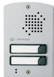
Audio push-button panels for 1 or 2-way applications, outside wall-mounted or back box versions. Ideal for installations in gate poles because of the reduced dimensions. Common technical features as all the range: front panel in anodised aluminium, led for name plate backlighting, amplified electric speaker. Back box included in the back box versions; rain shelter included in the surface-mounted versions. The UP11D, UP12D, UP111 and UP211 are only for kits 1+1 with alternate current call.
