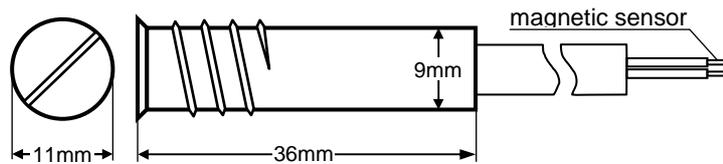
Fig. 3 Reed relay of K-3 magnetic contact in metal housing
