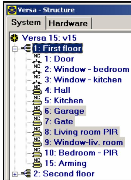
Fig. 6. List of partitions and zones in a tree-like form in the "System" tab, "Versa – Structure" window (an example of configuration).
