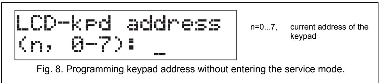
Fig. 8. Programming keypad address without entering the service mode.
