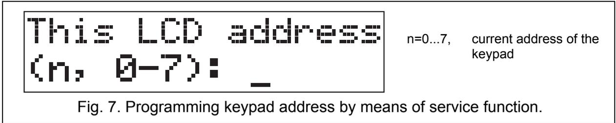
Fig. 7. Programming keypad address by means of service function.
