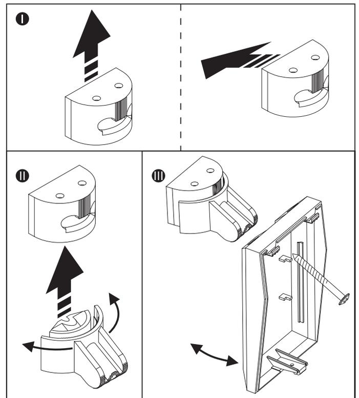
Figure 3. Mounting the detector on holder.
