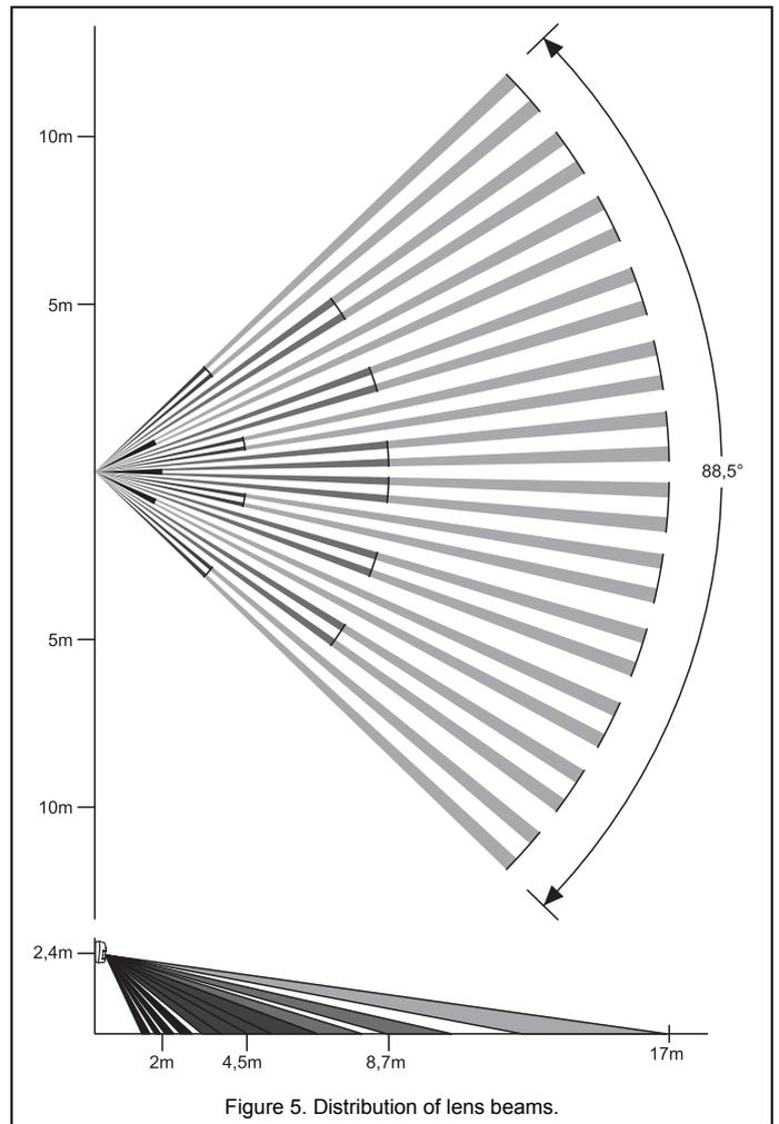
Figure 5. Distribution of lens beams.
