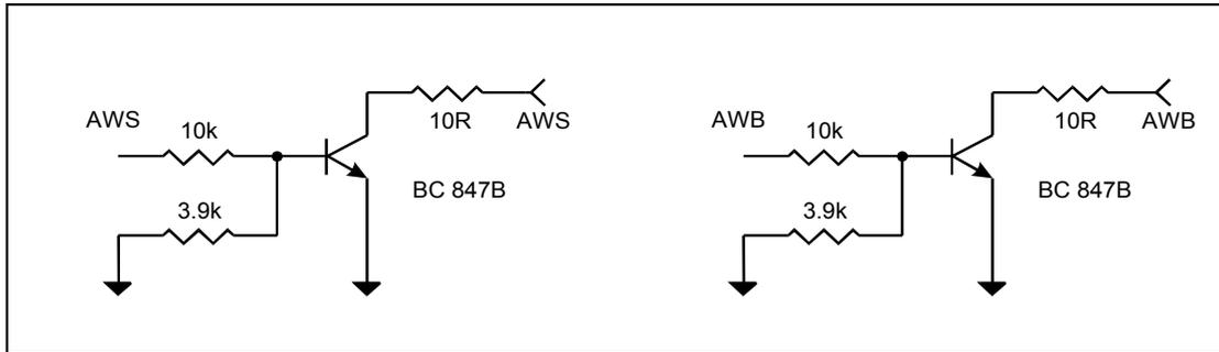
Figure 2. Schematic view of AWS and AWB outputs.
