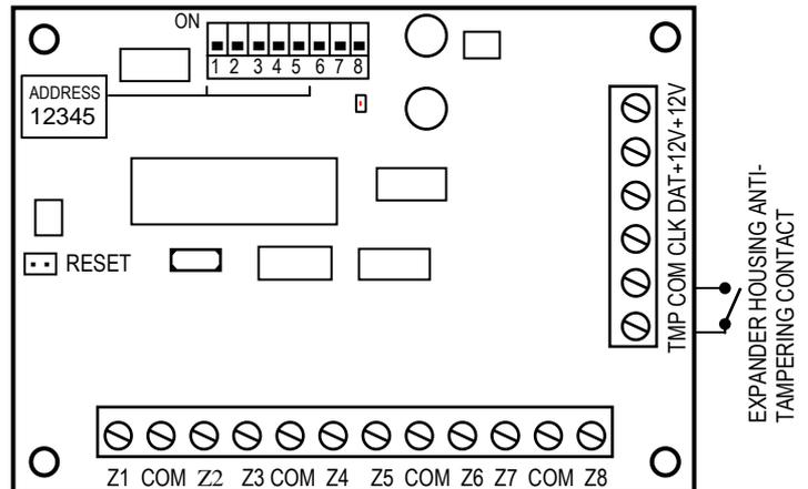
The **set of switches** situated on the board serves to set up the individual expander address. Up to 32 modules of various types can be connected to one bus. Six expander zones can be installed in the system, unless the zones in LCD keypads are used (the total - maximum - number of zones is 64).
