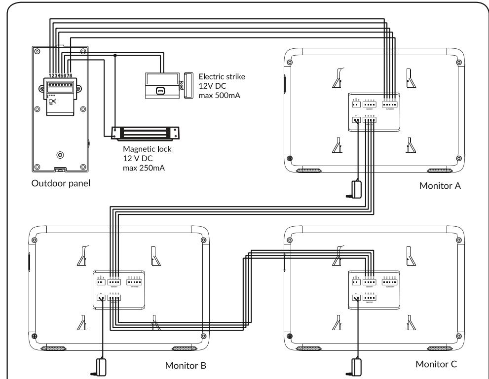
**Note:** Do not connect both the electric striker and the magnetic lock at the same time. Select only one type of closure.
