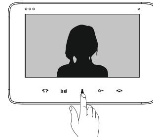
To preview the camera image, press the MONITORING button. Press the same button again to return to standby mode.
