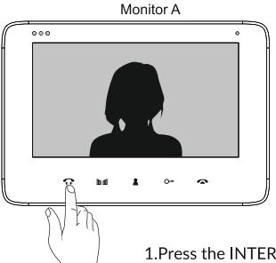
1. Press the INTERCOM button to start communication between the monitors.
