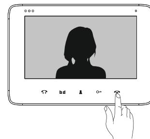
Monitoring time: approx. 40 seconds. After 40 seconds, the monitor will automatically return to standby mode.
