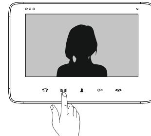
To open the outside gate, press the GATE CONTROL button.
