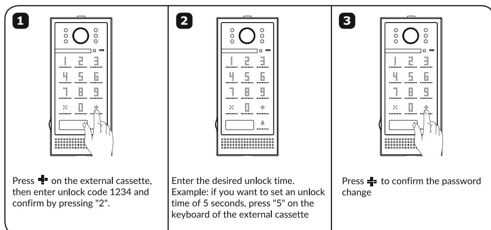
Press on the external cassette, then enter unlock code 1234 and confirm by pressing "2".
