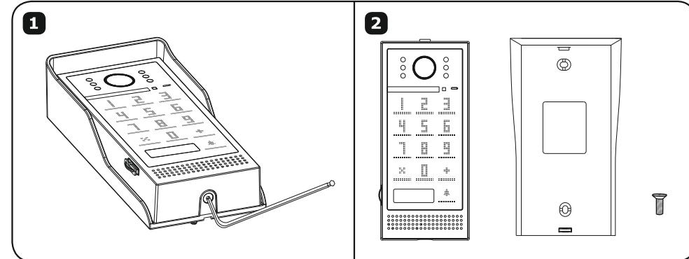
2. Fix the rain cover to the wall with screws.
