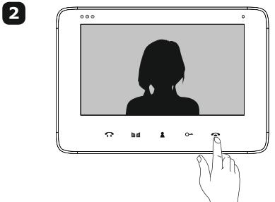
Press the TALK button to start a conversation with the person standing outside. Press the same button again to turn off the monitor panel.
