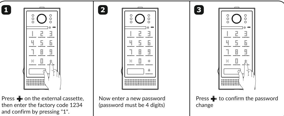
Press on the external cassette, then enter the factory code 1234 and confirm by pressing "1".
