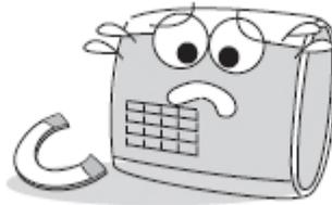
Do not place a magnet near the product. Magnetic objects such as a magnet, CRT, TV, monitor or speaker may damage the device.
